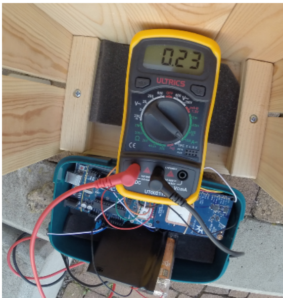
Figure 22 - Measuring energy consumption of the prototype with a multimeter set at 10A sensitivity to capture the initial large draw by the RockBLOCK
