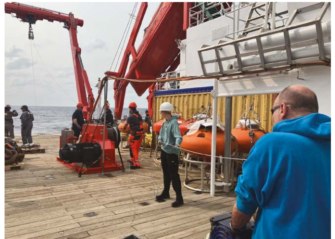
Crew and science team lower a mooring into the water via the A-frame at the stern of the ship. Image courtesy C. Mertens.
